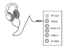
For private listening, connect headphone (not included) into the PHONES jack of TV. The speakers will be disconnected when headphone are inserted into the jack.
